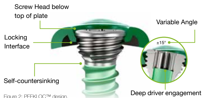
Figure 2: PEEKLOC TM design.
