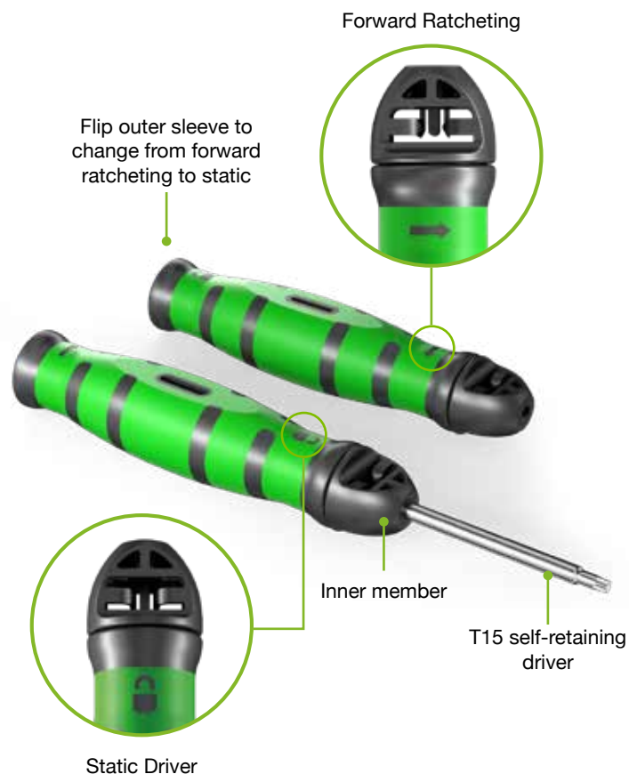
Figure 5: Ratcheting Handle – Illustration of its multifunctionality.
