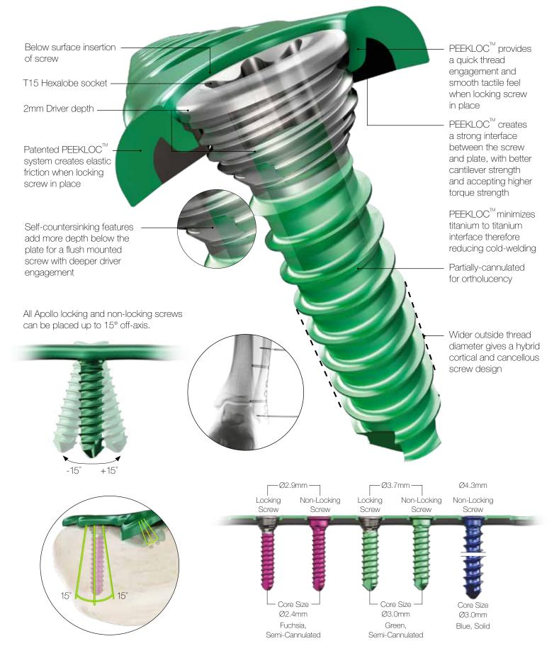
This thin cross-sectional structure of titanium gives the plates "ortholucency", a unique advantage over traditional metal implants where the radiolucent properties drastically improve the visualization of bones and joint spaces. Intraoperatively, surgeons benefit from improved fracture and joint reduction imaging, while postoperatively they can better assess if bone is healing properly, potentially leading to earlier weight bearing decisions.
